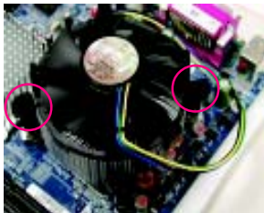
Fig. 3 Place the heatsink on top the CPU and make sure the push pins align to the pin hole on the motherboard. Push down the push pins diagonally.
