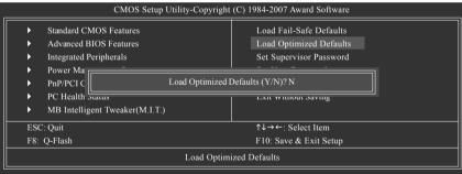
Selecting this field loads the factory defaults for BIOS and Chipset Features which the system automatically detects.
