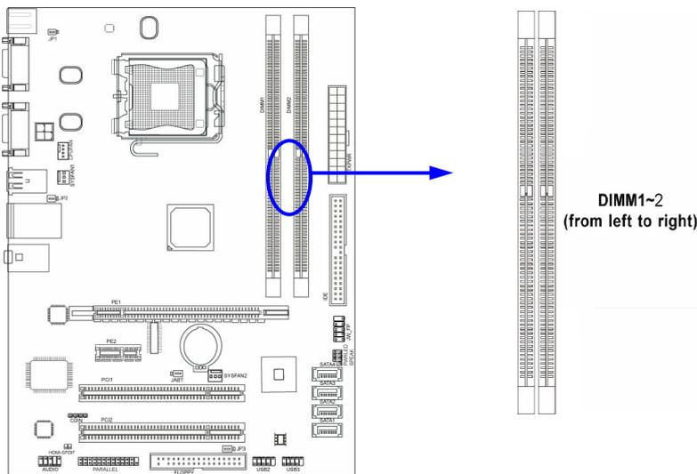
**NOTE!** When you install DIMM module fully into the DIMM socket the eject tab should be locked into the DIMM module very firmly and fit into its indentation on both sides.
