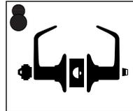
Turn/push-button locking; pushing and turning button locks outside lever requiring use of key until button is manually unlocked. Push-button locking: pushing button locks outside lever until unlocked by key or by turning inside lever.
