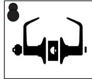
Push-button locking. Push-button locks outside lever until unlocked with key or by rotating inside lever.
