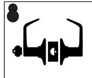
Outside lever locked and unlocked by key. Inside lever always unlocked.
