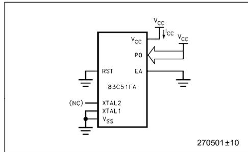
Figure 9.  $I_{CC}$  Test Condition,
