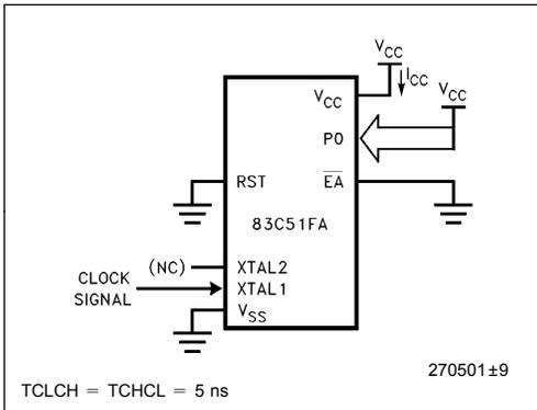
Figure 8.  $I_{CC}$  Test Condition Idle Mode.
