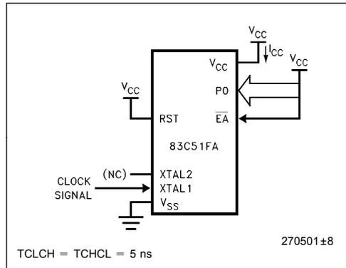
Figure 7.  $I_{CC}$  Test Condition, Active Mode
