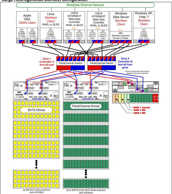
Example 1.Drawing depicts large and expandable SAN with heterogeneous client connectivity. Multiple DS5300 connected to meshed SAN fabric with a minimum of two Fibre Channel switches. For DS5100/DS5300 configurations, a minimum of two switches is recommended. Drawing shows multiple DS5300 for Data storage and a separate DS5020 for Meta Data.
