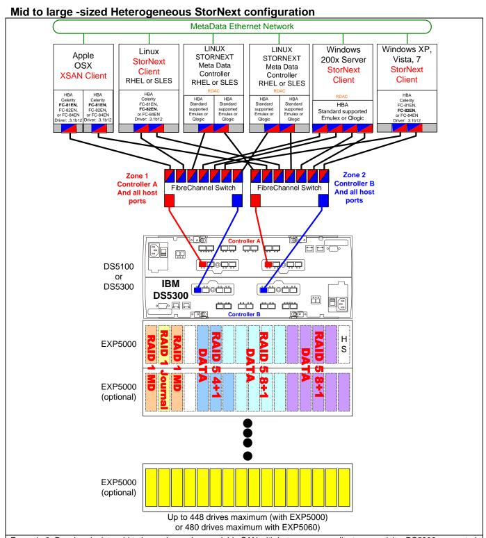
Example 6. Drawing depicts mid to large size and expandable SAN with heterogeneous client connectivity. DS5300 connected to meshed SAN fabric with a minimum of two Fibre Channel switches. For DS5100/DS5300 configurations, a minimum of two switches is recommended. Drawing shows minimal SAN to DS5300 connections to simplify the drawing. However, up to 16 connections is supported.
