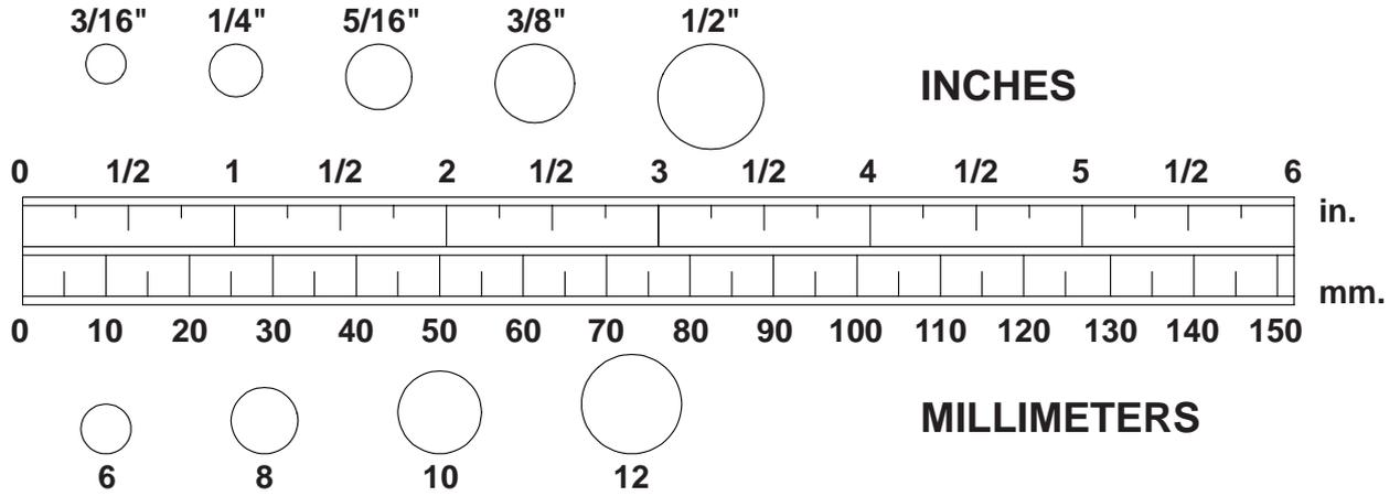
Place washers, the end of bolts or screws on the circles to check for the correct size. Use the small scale to check the sizes of bolts and screws.
