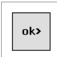
**OK Prompt:** Enables you to go directly to the Open Firmware command prompt. The Open Firmware command prompt is used for debugging and device driver development. For more information about the operation of the Open Firmware command prompt, refer to IEEE Standard 1275.
