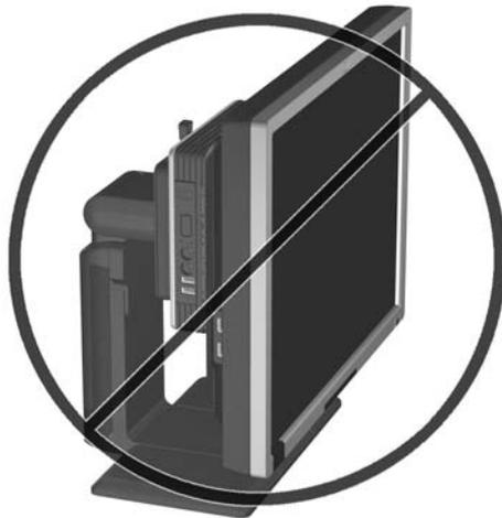
**Figure 5-9** Unsupported mounting position - thin client between stand and monitor
