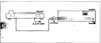
Connect the red plug to the right-channel jack (R), and the white plug to the left-channel jack (L).
