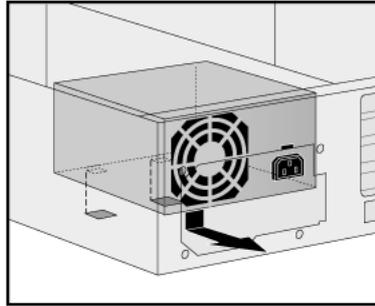
7 Replace the four screws to secure the power supply.
