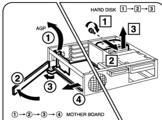
Shows how to remove the hard disk drive
