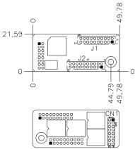
J1 J2: COM3/4/5/6 Serial Ports J1 - COM3/4 pin-header connector. PIN1~PIN10 COM3 PIN11~PIN20 COM4 J2 - COM5/6 pin-header connector. PIN1~PIN10 COM5
