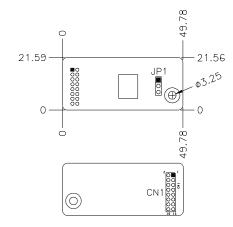
CN1: LPC I/F connectors Package list Nylon Nut x 1 Screw x 2 Washer x2
