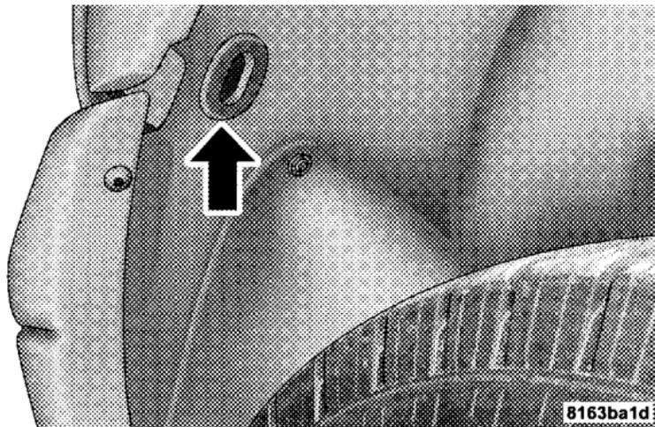
4. Remove the nut through the access hole.
