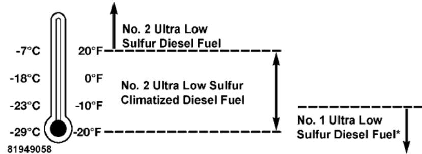
\*No. 1 Ultra Low Sulfur Diesel Fuel should only be used where extended arctic conditions (-10°F/-23°C) exist.
