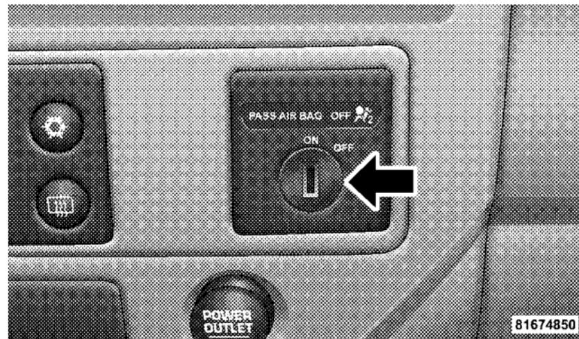
Passenger Airbag On/Off Switch
