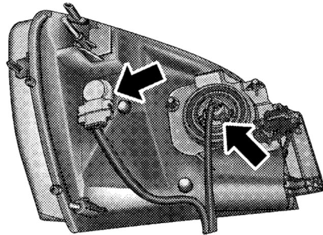
7. Twist connector on the side marker/turn signal/park lamp bulb  $\frac{1}{4}$  turn and remove connector and bulb from housing.
