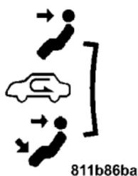
Select the recirculation modes when the outside air contains smoke or odors. This feature allows for recirculation of interior air only. Air flows through the panel outlets in this mode. Air flows through the panel only or through both the panel and floor vents depending on the selected mode (panel vs bi-level).
