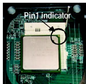
2. Locate Pin 1 in the socket and look for a (golden) cut edge on the CPU upper corner. Then insert the CPU into the socket.
