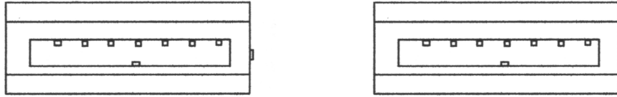
Figure 3: Using SeriTek/2SE2-E with a drive enclosure that has I-shaped eSATA connectors; both cable connectors will be identical.
