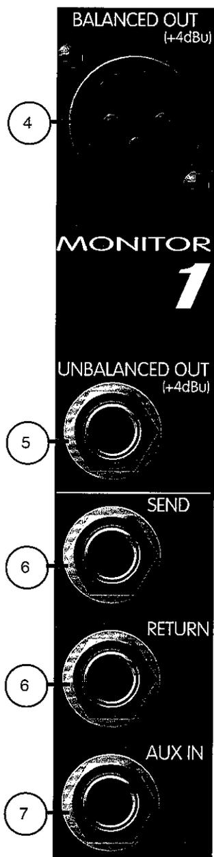
**4. Balanced Outputs:** The SRM is equipped with 1 XLR balanced output for **each** Monitor channel. This balanced output is +4 dBu. Connecting from this output to the balanced input of your monitor power amp is the preferred method of signal patching. The balanced output can be used simultaneously with the Unbalanced Output (#5).
