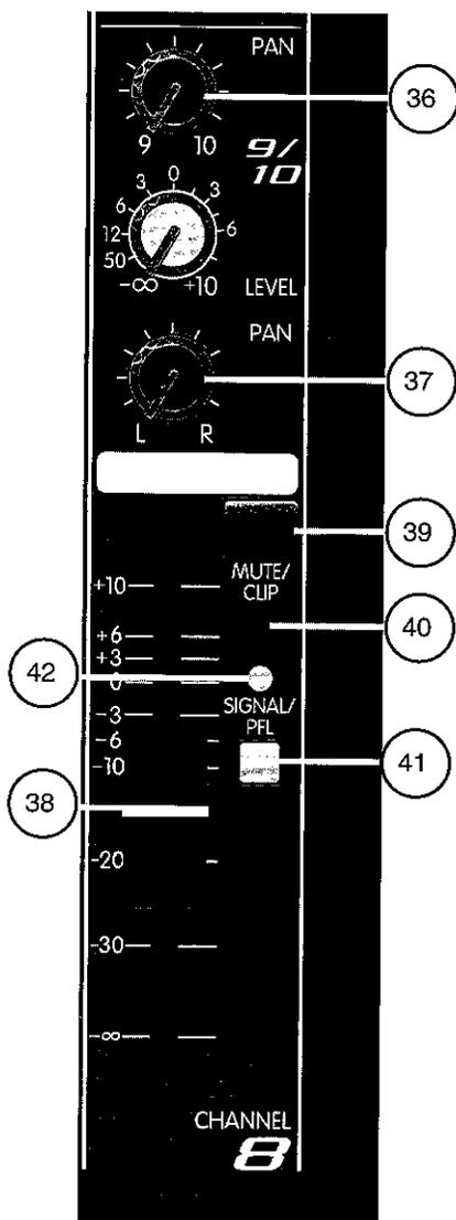
**36. 9/10 Pan:** This control sets the balance of the channel’s signal between Monitor Sends 9 and 10.
