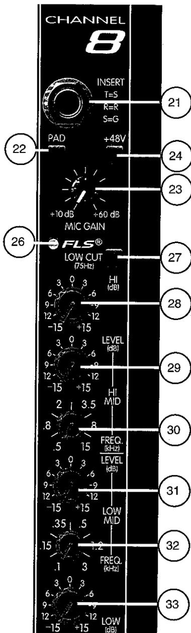
**21. Insert:** An Insert jack is provided to allow for an external device (i.e., compressor, effects, tuner, etc.) to be placed in the signal path pre EQ. The jack is wired: Tip=Send, Ring=Return, and Sleeve=Ground. A switch in the jack normally connects the Tip and Ring to continue signal flow when the jack is not in use. When a plug is inserted into the jack, the signal chain is broken and the signal must be properly returned.
