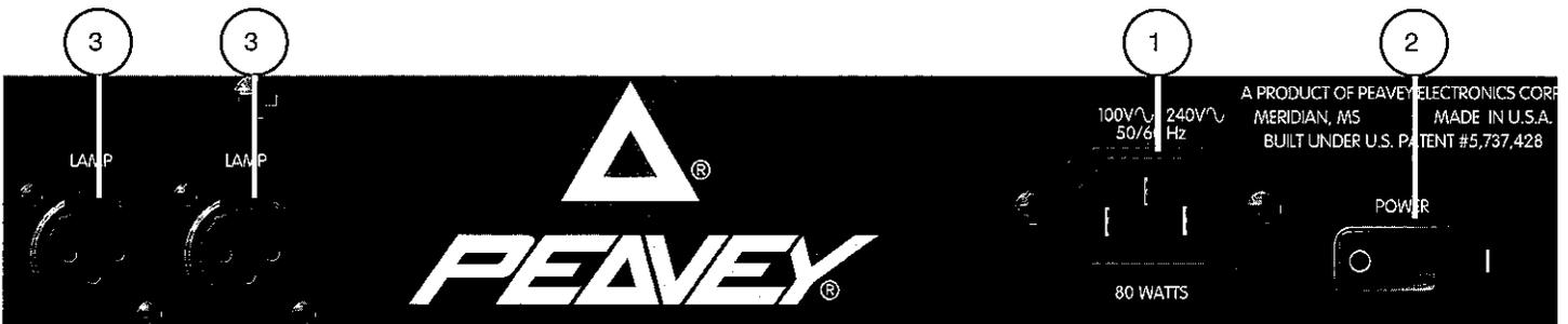
**1. IEC Power Socket:** With the Power Switch (#2) in the off (O) position, plug the power cord into this connector prior to plugging it into your AC power source. **Always insure that proper grounding practices are utilized.** Your SRM uses a universal switching power supply designed to operate with nominal line voltages ranging from 100 to 240 VAC. You may now plug the power cord into the AC power source.
