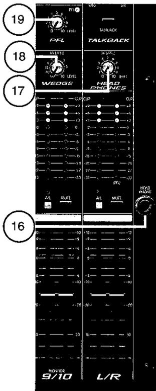
**16. Headphone Output:** This stereo jack (TRS) provides the signal to drive stereo headphones. No signal is heard until either AFL (#13) or PFL (#41) is selected on an active Master Monitor output. If both AFL and PFL are selected simultaneously from the same output, the PFL signal will be heard. The stereo jack is wired: Tip=Left, Ring=Right, and Sleeve=Ground.
