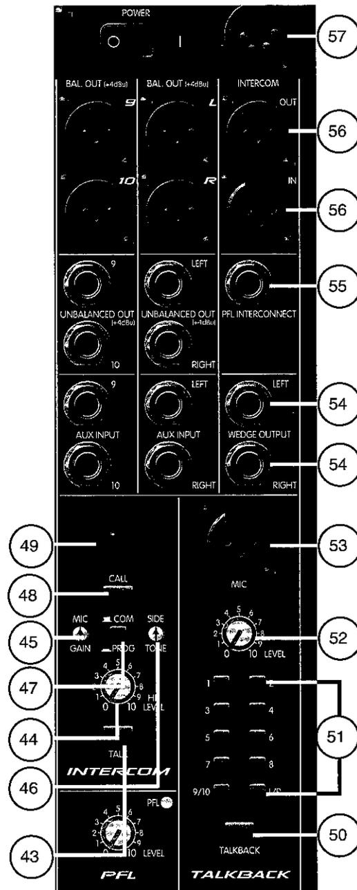
**43. Talk:** Press this momentary switch to speak through the headset microphone and onto the intercom line. The mic level is adjusted by the Mic Gain trim pot (#45) and the amount of your mic signal fed back into your headset is adjusted by the Side Tone trim pot (#46).
