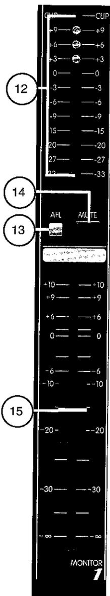
**12. LED Peak Level Meters:** Each of the 12 monitor mixes has a 12 segment LED Peak Level Meter with a -33 to +9 dB range. Each meter has a clip warning LED to indicate when the signal is within 2 dB of clipping. The 0 dB reference level of all meters corresponds to +4 dBu at its output. The R Meter (furthest to the right) is also used with priority for PFL metering.
