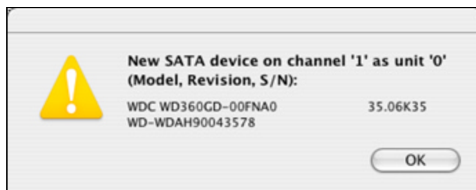
Figure 16: Example Serial ATA hard drive connected to channel 1
