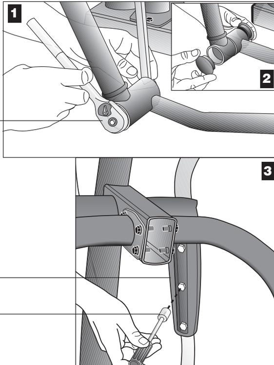
e. Wrench tighten using a  $\frac{9}{16}$ -inch socket and open end wrench. Refer to Diagram 15, #1.
