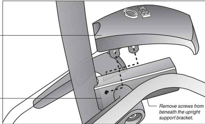
20. **Attach the bracket cover.** Diagram 16. Take the following steps to attach the cover over the upright support bracket.
