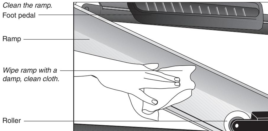
22. **Clean the ramp.** Diagram 18. Wipe down the ramp and foot pedals with a soft cloth dampened in a diluted solution of mild soap and water.
