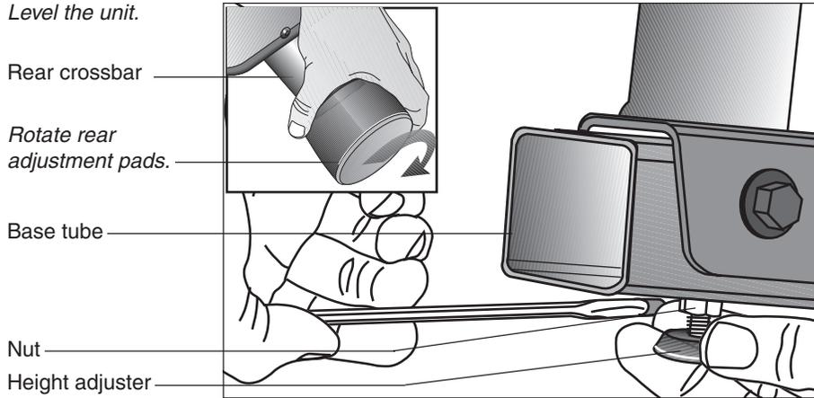
21. **Level the unit.** Diagram 17. To keep the unit stable, the EFX has adjustable rear pads and, at the front of the base assembly, a height adjuster. Check to make sure that the unit does not wobble from side to side or front to back.
