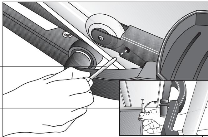
The locking pin secures the roller arm and keeps it from traveling up or down the ramp. Pull firmly on the pin to slide it out of the ramp. A lanyard is attached to the locking pin and ramp. Refer to Diagram 20.
