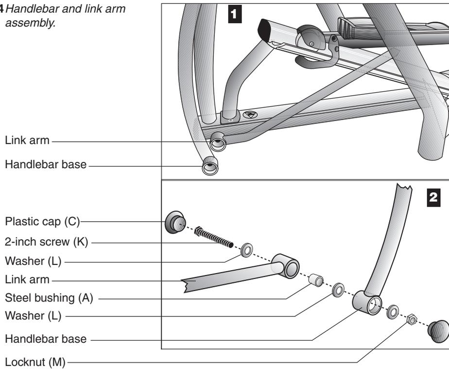
b. Thread screw (K) with washer (L) through the link arm. Refer to Diagram 14, #1 and #2.
