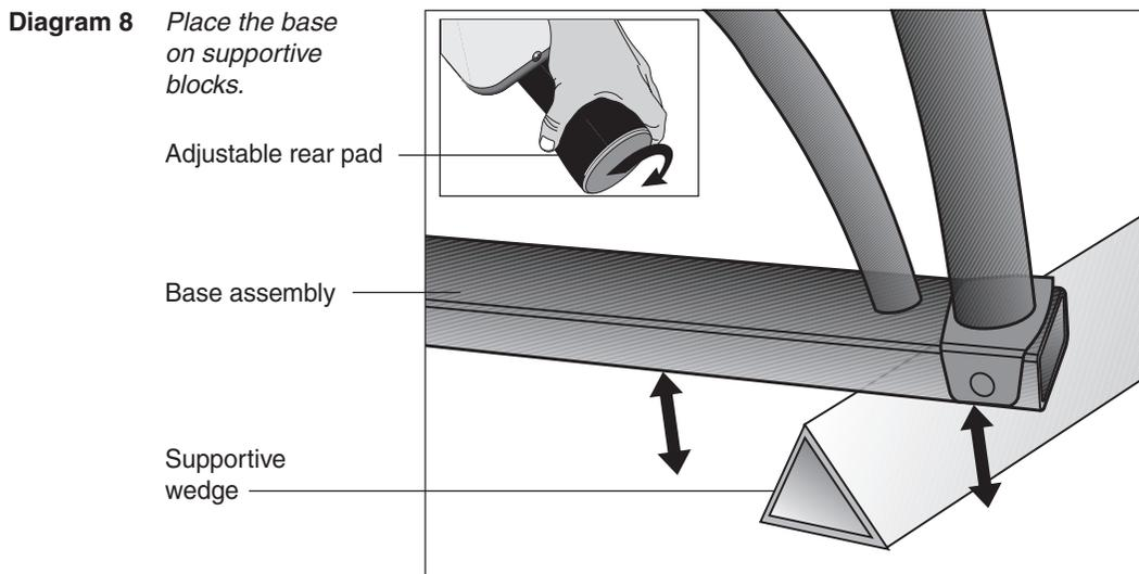
12. **Rotate the rear pads.** Diagram 8, inset. Ask your assistant to stabilize the unit while you rotate the rear adjustable pad to the highest position. This procedure lifts the base assembly off the floor which provides better access to the fasteners.
