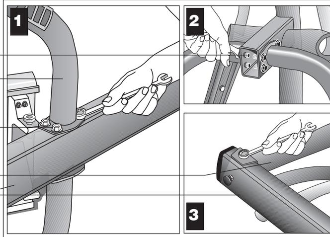
**15. Tighten all mounting screws using a 9/16-inch wrench.** Diagram 11.
