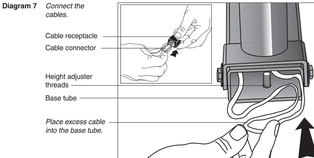
10. **Connect the cable.** Diagram 7, inset. Insert the cable into its receptacle. Just like a telephone connection, a definite "click" is heard when a good connection is made. If you do not hear a "click," try reinserting the cable connection again.
