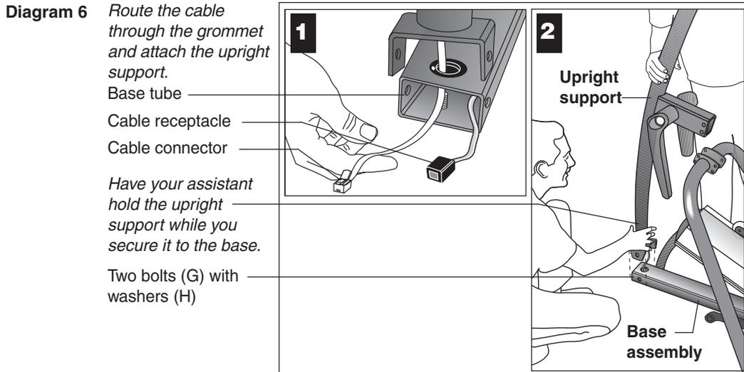
8. **Position the upright support over the base.** Diagram 6. Have your assistant move the upright support close to the front of the base assembly while you thread the cable through the grommet hole and out the front of the base tube (see inset #1). Make sure that the display console (on the upright support) faces the rear of the unit (see inset #2).
