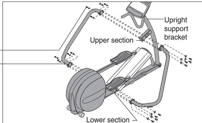
14. **Attach the left and right frame stabilizers.** Diagram 9. Proceed with one side at a time. When you have installed the first stabilizer, perform the same steps on the opposite stabilizer.
