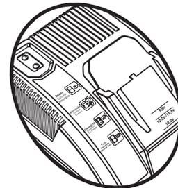
**NOTE:** The 9.6 Volt, 12 Volt, and 14.4 Volt battery packs will not slide all the way down onto the charger port. Insert 9.6 Volt, 12 Volt, and 14.4 Volt battery packs until they click into place and are aligned with the line on the charger, shown at left.
