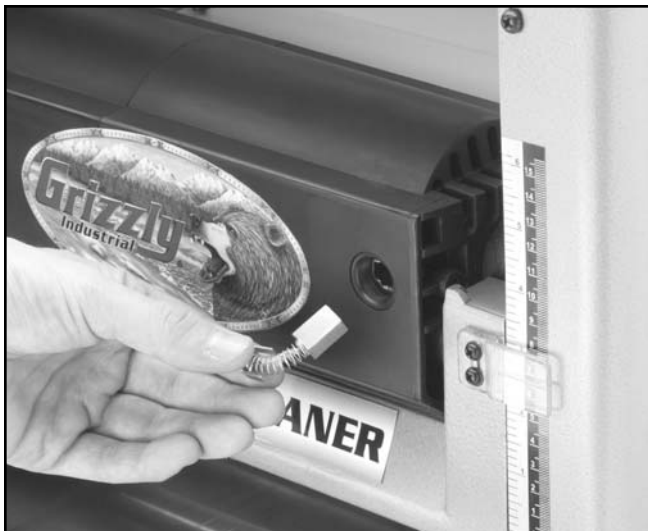
Figure 10. Brush holder location (another brush is located on the other side of the motor from the one shown in this picture).
