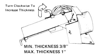
Thickness of the ice can be varied by rotation of the inverted "L" shaped adjusting screw which is located on the thickness control. The thickness control is mounted on the lower freezing plate. One complete rotation of the adjusting screw varies the thickness approximately 1/16". To increase thickness turn the screw in a clockwise direction. Maximum production of ice in pounds will be obtained with the control set to produce ice approximately 1/2" thick.
