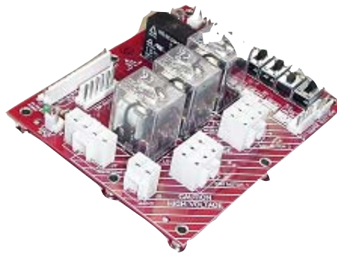
Figure O-GI-1. Relay board
