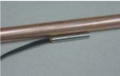
Figure I-MR-4. Close-up view of the changeover sensor
