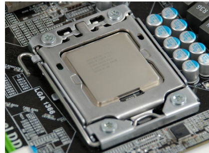
Align notches with notches on the CPU
