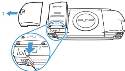
Align the tabs, and then slide the cover in the direction of the arrow until it locks firmly in place.
