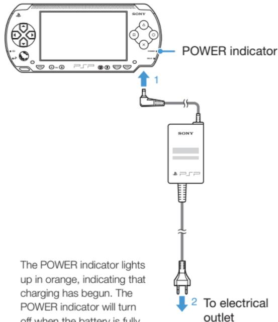
The POWER indicator lights up in orange, indicating that charging has begun. The POWER indicator will turn off when the battery is fully charged.
