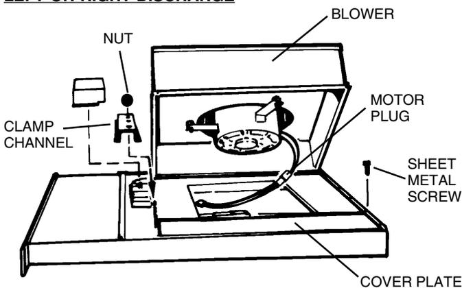
1. Remove the 4 nuts and 2 clamp channels.
