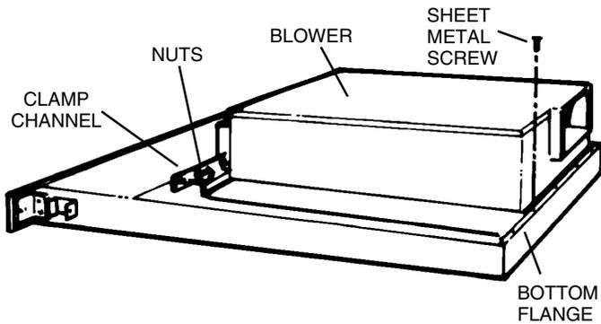
1. Loosen the 4 nuts and 2 clamp channels.
