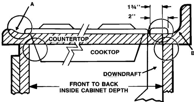
Pay special attention to the areas of potential interference highlighted above. A countertop with (A) a raised lip and/or (B) a backsplash may not allow enough flat countertop for a proper installation. Note that 2" of flat countertop is required behind cooktop and that 1-3/4" is necessary between the back edge of the cooktop and the inside of cabinet back.
