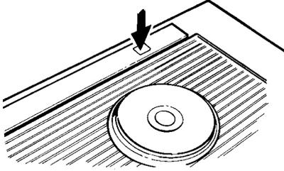
Turn the downdraft blower ON by pressing down on the activating switch. The air vent will rise.
