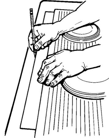
3. Place the plastic template against the back flange of the cooktop and center it. Trace around template to mark the downdraft opening.
