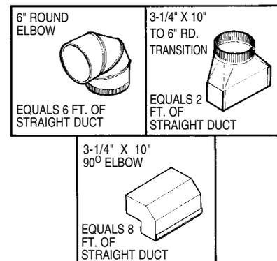
3. The system will operate most efficiently when the ductwork does not exceed 40 feet of equivalent duct. The chart, above, shows equivalent feet of elbows and transitions. The number of feet of straight duct plus the equivalent feet of transitions and/or elbows to be used should equal 40 feet or less.
