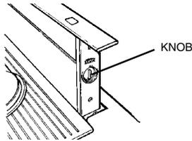
The blower can be turned ON or OFF and its speed can be adjusted with the recessed knob on the right side of the air vent.
