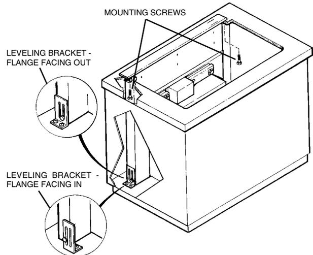
1. Set downdraft into opening. Extend leveling brackets to floor of cabinet so downdraft sits straight. (Note: Leveling brackets can be removed and re-attached in other positions. Bottom flange may have to face inward in tight cabinet installations.)
