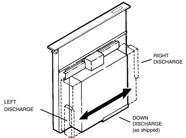
1. This downdraft blower system is designed for use with 3-1/4" x 10" ductwork (can be transitioned to 6" round). Three different discharge directions are available with side-to-side adjustment for accurate alignment of ductwork.
