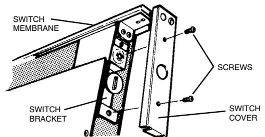
3. Remove switch cover from right end of air vent.
