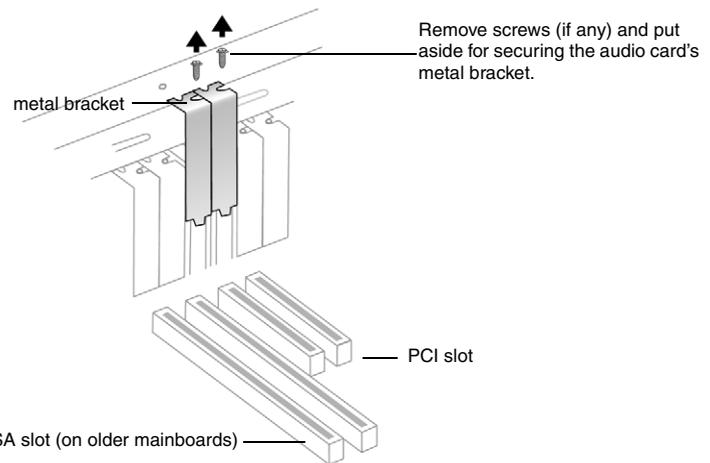
Figure 2-2: Removing metal brackets
