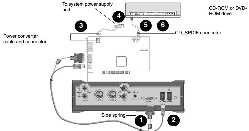
Figure 2-5: Connecting the cables to the audio card.
