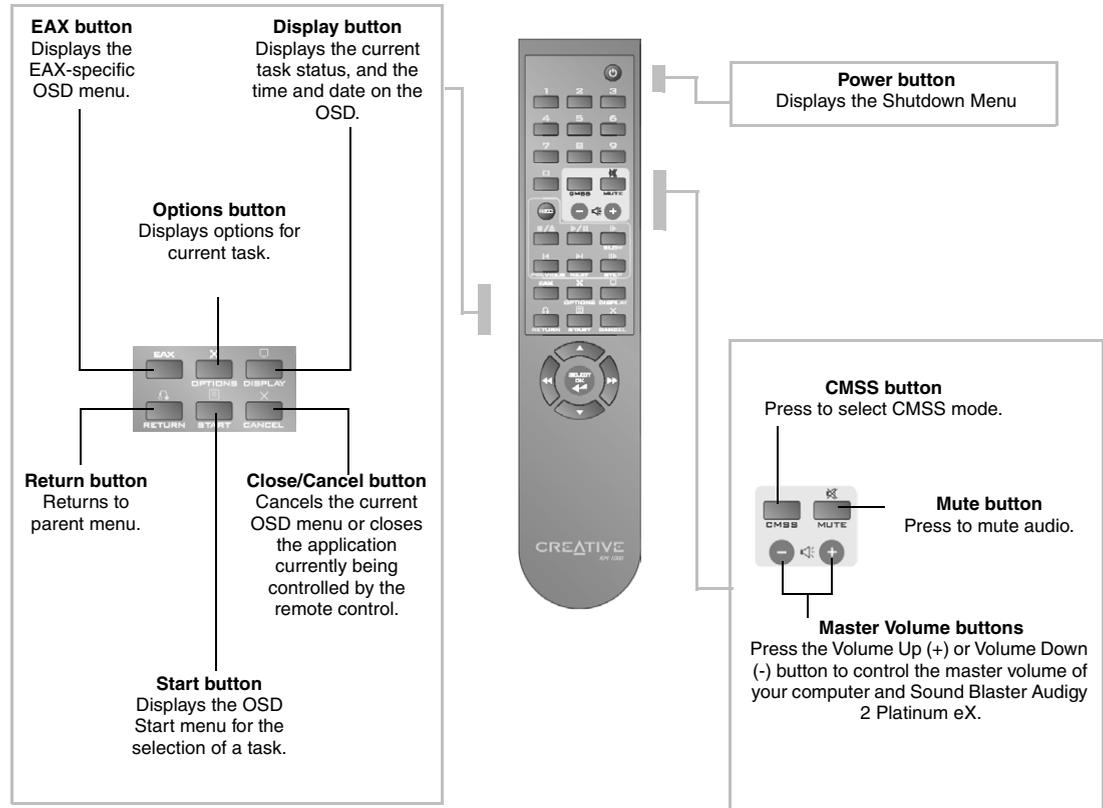
Figure 1-5: Other Buttons on the Remote Control.
