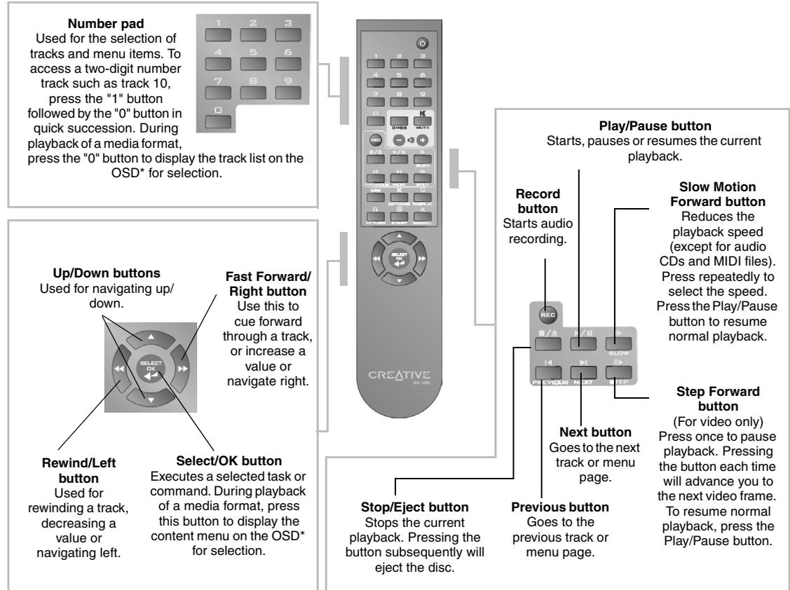
Figure 1-4: Navigation Buttons on the Remote Control.
