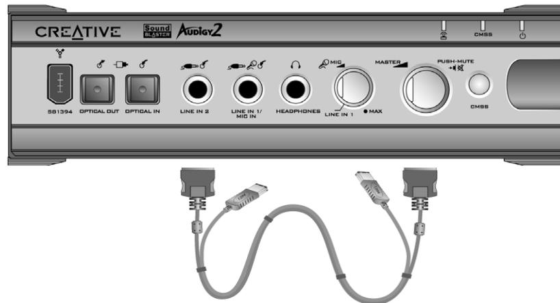
Figure 2-1: Audigy 2 Platinum eX External I/O Module and AD\_LINK cable
