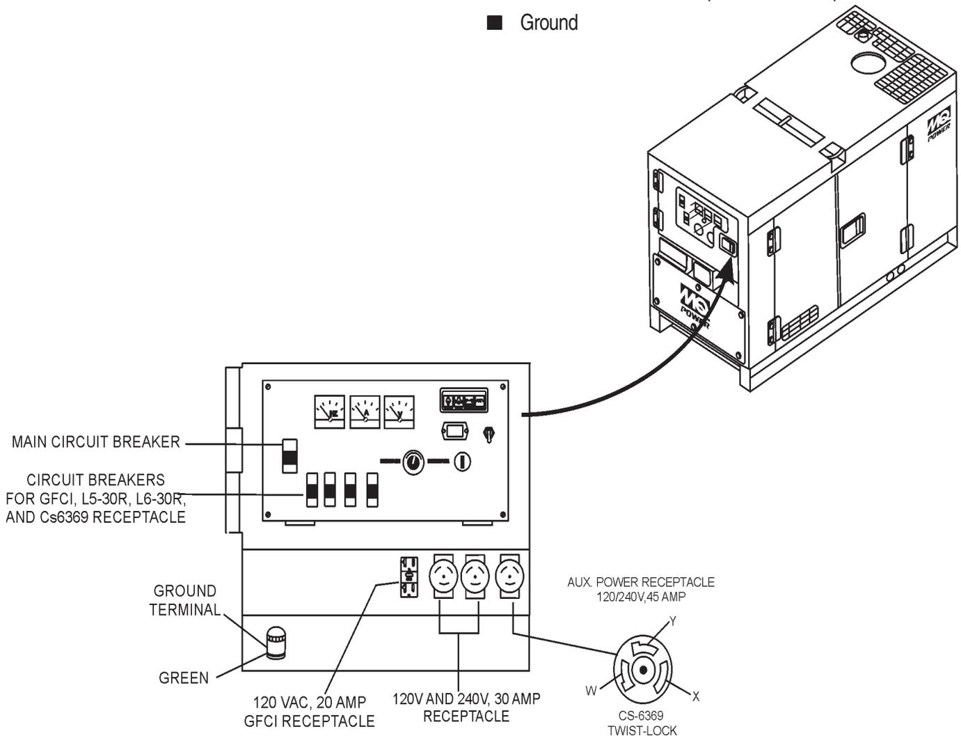
Figure 5. Output Terminal Panel
