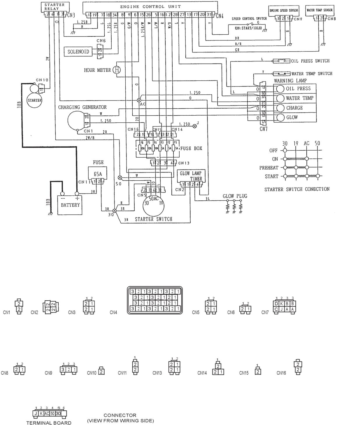
Figure 35. Engine Wiring Diagram
