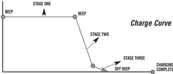
**Stage Three** — Top-Off Charge voltage is automatically maintained and reduced to a predetermined level while current is adjusted for a safe, effective battery charge. At the end of Stage 3, the unit will BEEP signaling the completion of the charging cycle.
