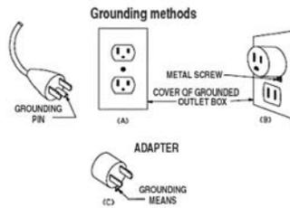
The battery charger is for use on a nominal 120 volt circuit, and has a grounding plug that looks like the plug illustrated in Figure A. A temporary adapter, which looks like the plug illustrated in Figures B and C may be used to connect this plug to a two-pole receptacle as shown in Figure B if a properly grounded outlet is not available. The temporary adapter should be used only until a properly grounded outlet can be installed by a qualified electrician.
