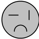
Figure 3-1. Tandem Prong-type Plug
