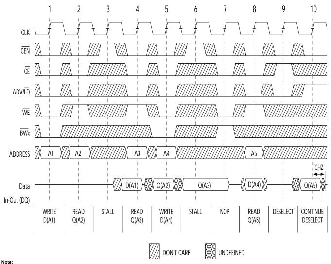
26. The IGNORE CLOCK EDGE or STALL cycle (Clock 3) illustrated CEN being used to create a pause. A write is not performed during this cycle.
