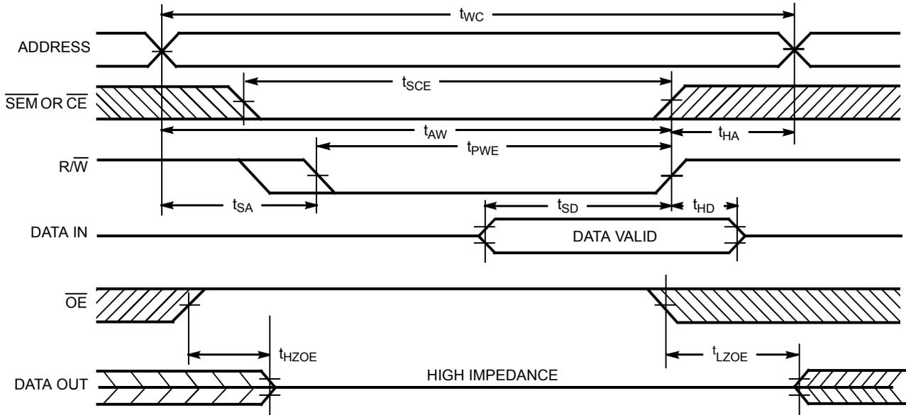
Figure 7. Write Cycle No. 2: R/W Three-States Data I/Os (Either Port)<sup>[22, 24, 25]</sup>
