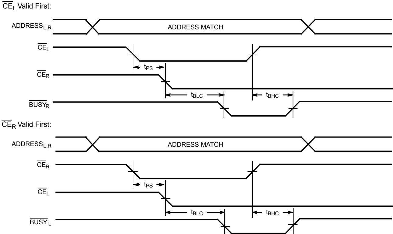
Figure 13. Busy Timing Diagram No. 2 (Address Arbitration)<sup>[30]</sup>
