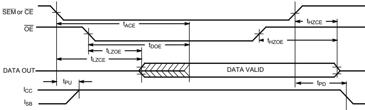
Figure 5. Read Timing with Port-to-Port Delay ( $M/\bar{S} = L$ )<sup>[20, 21]</sup>
