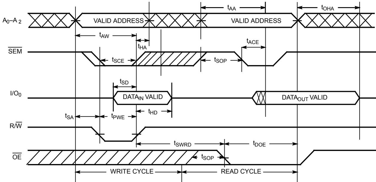
Figure 9. Timing Diagram of Semaphore Contention<sup>[27, 28, 29]</sup>
