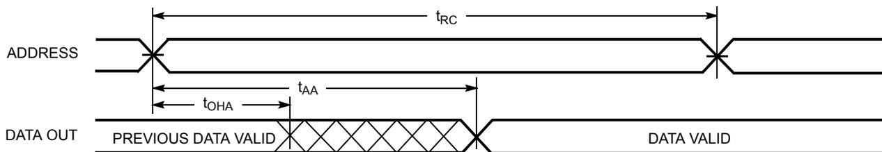
**Figure 4. Read Cycle No. 2 (Either Port CE/OE Access)<sup>[16, 18, 19]</sup>**
