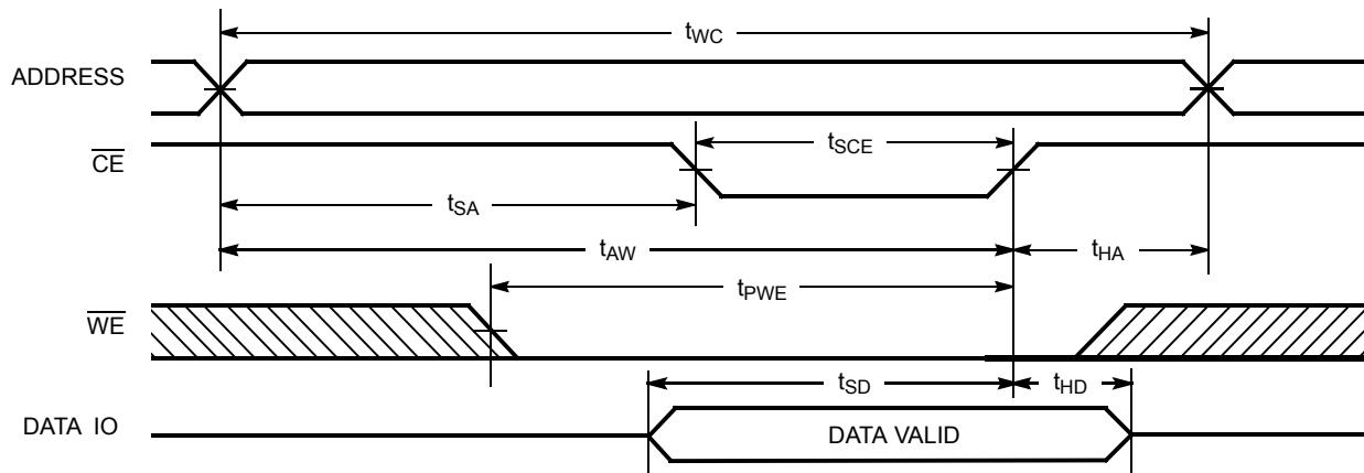
**Write Cycle No. 2 ( $\overline{\text{WE}}$  Controlled,  $\overline{\text{OE}}$  HIGH During Write) [18, 19]**
