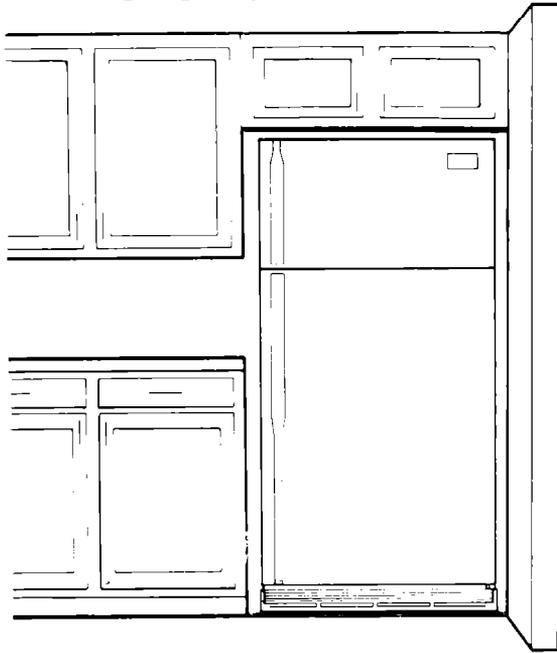
1. Allow  $\frac{1}{2}$ " (.2 cm) space on each side and at top for ease of installation.
