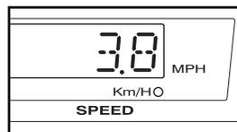
of the walking belt as desired by pressing the Speed + and – buttons. Each time a button is pressed, the speed setting will change by 0.1 mph; if a button is held down, the speed setting will change in increments of 0.5 mph.
