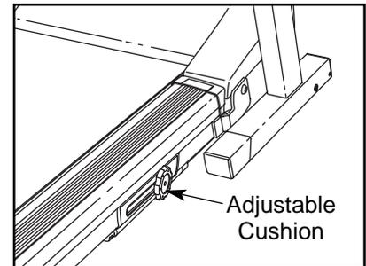
**Note: The faster you run on the treadmill, or the more you weigh, the firmer the cushioning system should be.**
