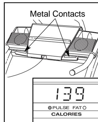
When your pulse is detected, the Pulse indicator will light and then your heart rate will be shown in the main display. **For the most accurate heart rate reading, continue to hold the contacts for about 15 seconds.**
