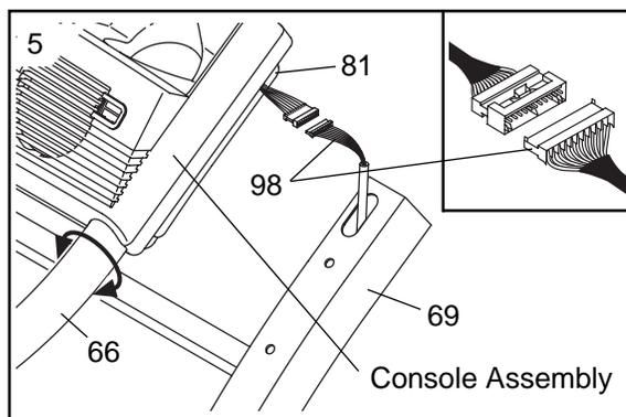
6. Insert two Handrail Bolts (78) with 5/16" Star Washers (77) into the right Upright (69) and the right Handrail (66). **Be careful not to damage the Upright Wire Harness (not shown).** Next, lift the right Handrail slightly and align the Bolts with the holes in the Handrail. (Note: If necessary, twist the Handrail to align the holes in the Handrail with the Bolts). Thread the Bolts into the Handrail. **Do not tighten the Bolts yet.**
