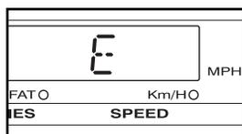
To reset the main display, press the Stop button, remove the key, and then reinsert the key.
