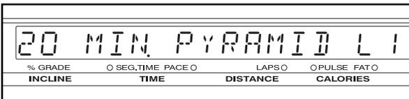
Three seconds after a preset program is selected, the name of the selected program, the maximum speed setting for the program, the maximum incline setting for the program, and the total program time will begin to scroll across the main display.
