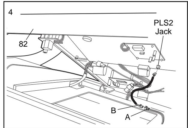
**Make sure that no wires are pinched.** See step 2. Reattach the Console (81) with the screws. **Important: If the screws are not put back into the same holes from which they were removed, the Console will be damaged.**
