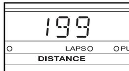
An "E" for English miles or an "M" for metric kilometers will appear on the right side of the main display. Press the Speed + button to change the unit of measurement.
