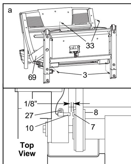
Locate the Reed Switch (10) and the Magnet (7) on the left side of the Pulley (8). Turn the Pulley until the Magnet is aligned with the Reed Switch. **Make sure that the gap between the Magnet and the Reed Switch is about 1/8"**. If necessary, loosen the Screw (27) and move the Reed Switch slightly. Retighten the Screw. Reattach the hood, making sure the screws are in their same holes. Run the treadmill for a few minutes to check for a correct speed reading.
