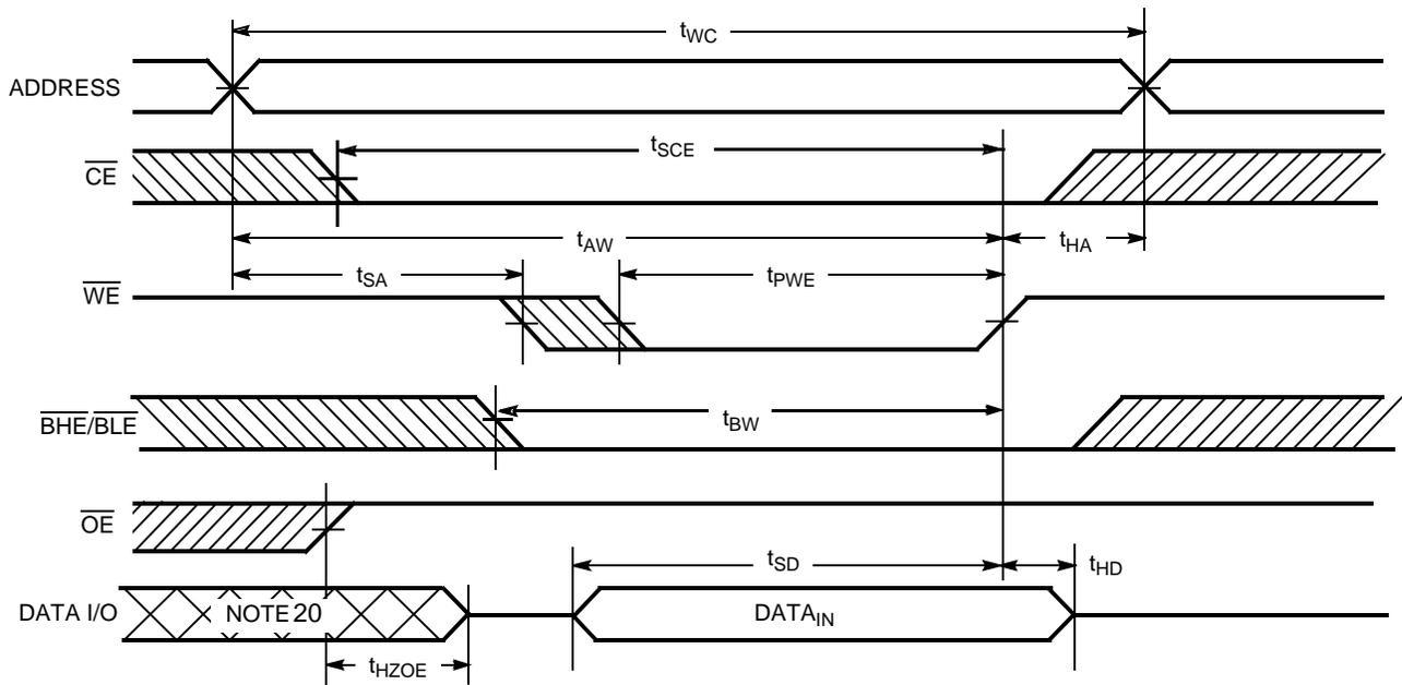
Write Cycle No. 2 ( $\overline{CE}$  Controlled)<sup>[14, 18, 19]</sup>
