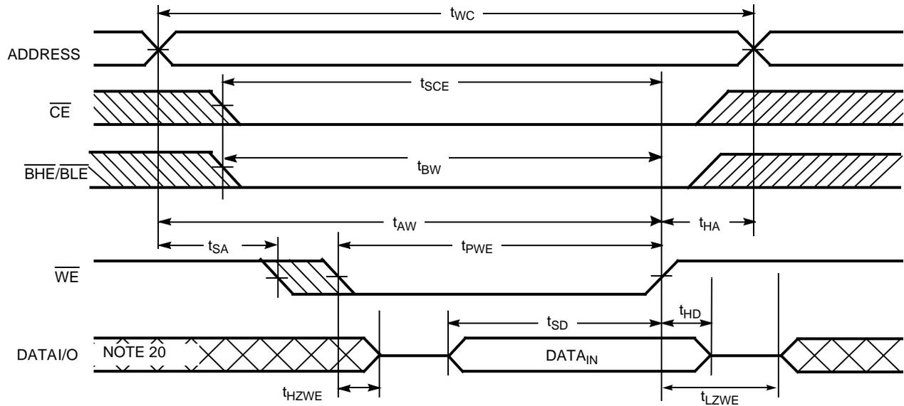
Write Cycle No. 4 ( $\overline{BHE}/\overline{BLE}$  Controlled,  $\overline{OE}$  LOW)<sup>[19]</sup>
