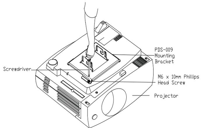
1. Invert the projector and place it on a soft and flat surface. Remove any foot levelers that might possibly prevent the correct installation of the bracket.
