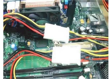
*The connected cables for two PL-P3/SMPs.*
