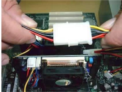
*Connecting the 4-pin end of the PL-P3/SMP's power cable to an unused 4-pin connector from the power supply.*
