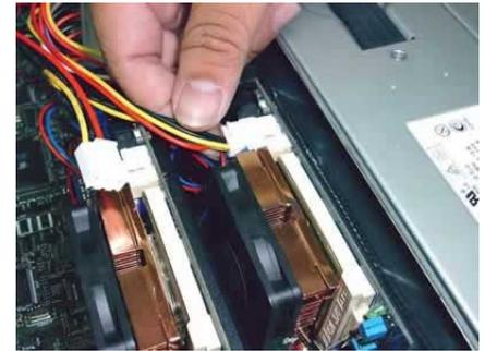
Connecting the power cable to the first PL-P3/SMP.
