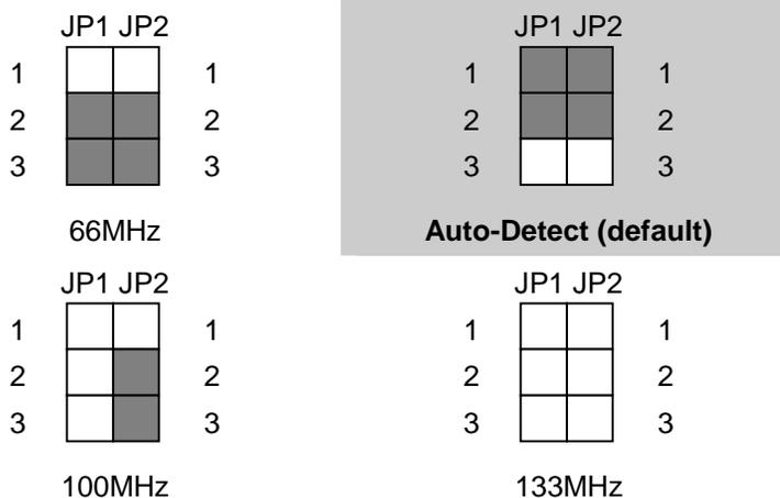
**Note:** This setting depends on the motherboard circuitry design: some VIA 694 chipset-based SMP motherboards can only work stably at 100MHz, not 133MHz.
