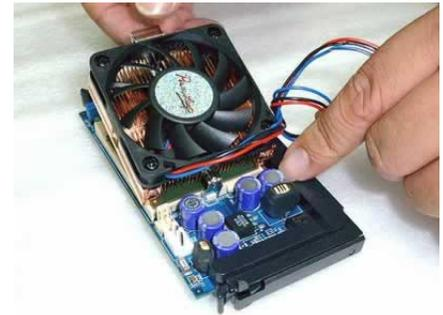
Installing the heatsink/fan onto the processor.
