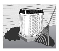
Efficiency can be maintained by keeping outdoor unit clear of debris, leaves and shrubbery.
