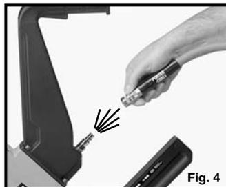
**9. DISCONNECT TOOL FROM AIR SUPPLY HOSE** before doing tool maintenance, clearing a jammed fastener, leaving work area, moving tool to another location, handing the tool to another person, or making adjustments. Fig. 5.
