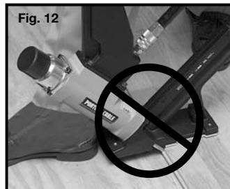
**23. DO NOT DRIVE FASTENERS** on top of other fasteners: the fasteners can ricochet causing personal injury.
