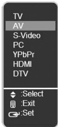
To change the Main Picture source, press the Input button on the remote to display the Main Picture (MP) input menu. When the input menu is on, use the up/down arrows to scroll through all inputs and the press enter to switch to the highlighted one.
