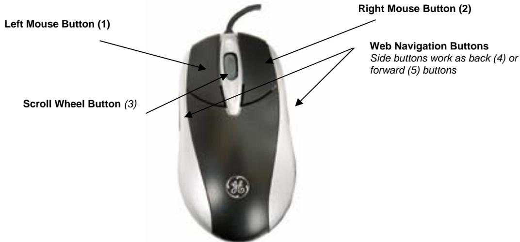
3. Scroll Wheel and Button – In applications that support it, roll the scroll wheel to move up or down. The scroll wheel also doubles as a third button. By default, this button activates or deactivates scroll lock. This feature allows any movement of the mouse to scroll through your document. This button can also be programmed to any one of 47 common functions using the included mouse software.
