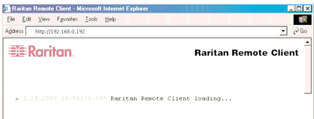
4. Raritan Remote Client (RRC), the applet used to access and control servers connected to Dominion KX, will automatically launch and display all Dominion KX units located on the same network subnet. If your Dominion KX unit is not automatically detected, select Connection > New Profile in the menu bar to create a new entry.
