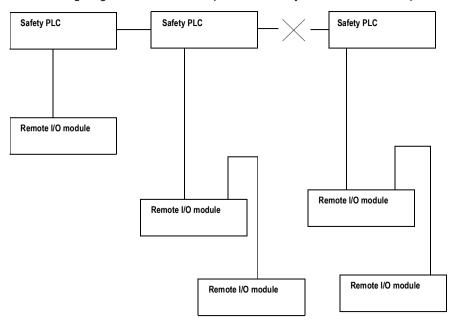
If the local network is reacting only on the inputs of the same system, the PLC system continues to run without failure.
