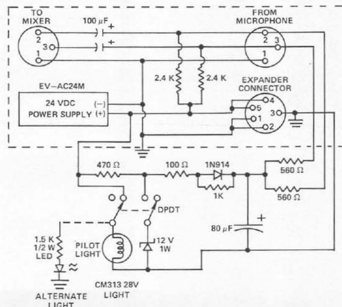
FIGURE 7 – Remote "Q" Light Activation Circuit
