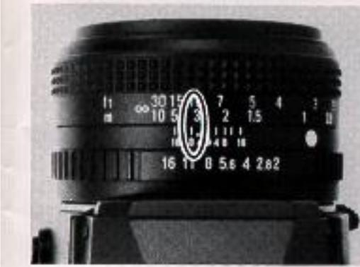
\* Infrared light rays are invisible to the eye and the light meter, so please refer to the instructions with the film for setting the f-stop number and shutter speed.....
