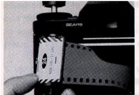
2. Insert the film in the Film Chamber and push the Film Rewind Knob down to its former position.
