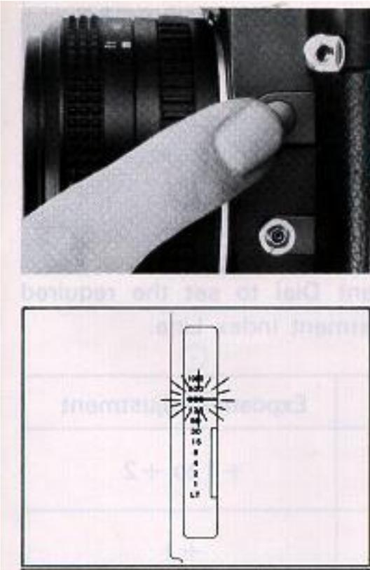
1. Move up close to the subject to measure the exposure, and press the AE Lock. The Shutter Speed Indicator in the viewfinder will pulsate to indicate that the exposure is locked onto the subject.
