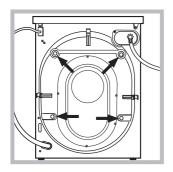
3. Remove the 4 protective screws and the rubber bush with the respective spacer, situated on the rear of the appliance (see also the installation leaflet). **NB:**The plastic spacers may fall down inside the machine once the bolt
