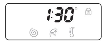
Once you have pressed the START/RESET button to start the programme, the display will indicate the amount of time left until the end of the wash cycle. If a delayed start has been set (using the Delay Timer, see page 9), the delay time will be indicated on the display.
