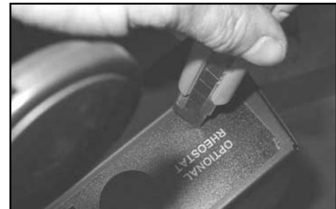
Figure 8.30 Reinstall rear shield. Connect blower to power supply and turn on gas supply.
