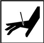
**Do not load nails with the trigger or safety depressed.** Unintentional firing may occur. Do not load nails when the air hose is connected to the tool. Always assume that the tool contains fasteners.
