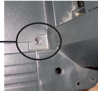
4. Position the rack right-side up (side panel locks at top) and drop the top panel onto the top of the rack. Fasten to the frame using M6 hex screws and the smaller Allen Wrench.
