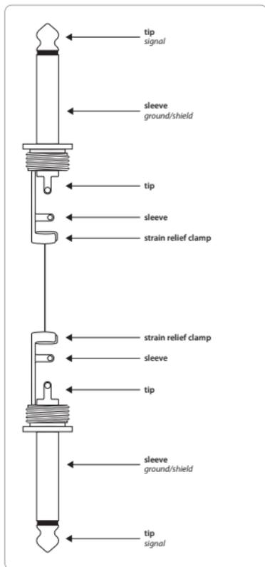
Fig. 5.1: Unbalanced jack cable with 1/4" TS jack plugs
