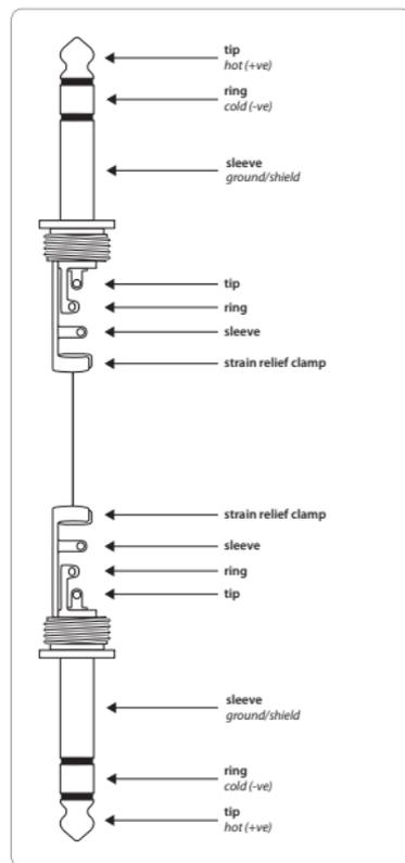
Fig. 5.2: Balanced jack cable with 1/4" TRS jack plugs
